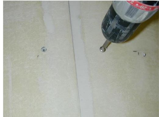
3) Reinstall pan head screws on the column half just assembled with adhesive.
