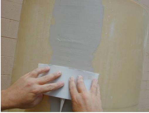
5) Smooth the body filler into a smooth radius using a thin sheet of plastic.
