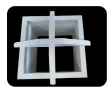
Apply adhesive to the flat cap part in the cut line (shown as open in photo below) then tape around the part to pull it square.
